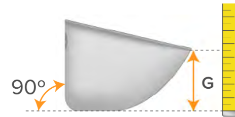
Measure the bucket edge Height "G"
