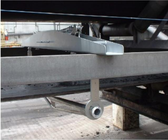
LB Belt Lifters deliver a reliable and efficient solution for all your belt lifting requirements. Specially designed to make roller replacement a simple and easy operation, reducing risk of injury to the operator or damage to the conveyor belt.
